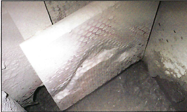
Transfer Point Deflector Liner shown above.
