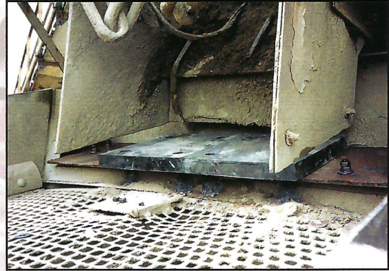
Custom made rubber feed lip liner
