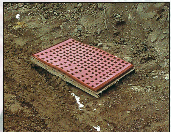
Hooked screen with impact zone.
